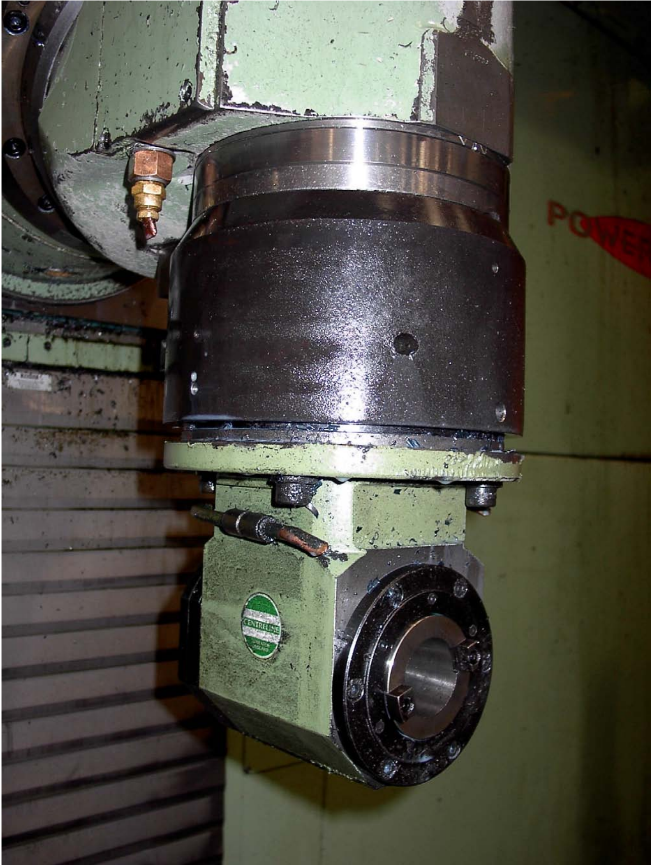
Large Right Angle Head Installed on Asquith Butler Machine at JCB Works, Cheadle, UK.
